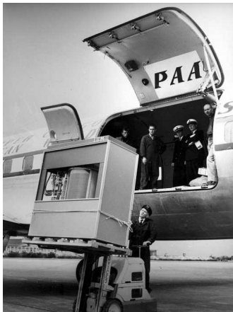
5MB hard drive 1956 (IBM RAMAC)
