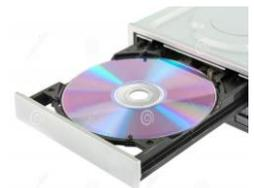
CD's are simply stamped (to form the pits) from a master and therefore relatively cheap to produce. CD-ROM disks provide a cheap form of mass storage storing approximately 650Mb. For example, a standard encyclopedia could be stored on a single CD-ROM. While 650Mb seemed quite large, it is now becoming smaller. Particularly when computers are using computers with hard disk storage of 10 or 20 Gigabytes.
