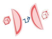
A device that uses concave mirrors to create the illusion of a 3D object.
