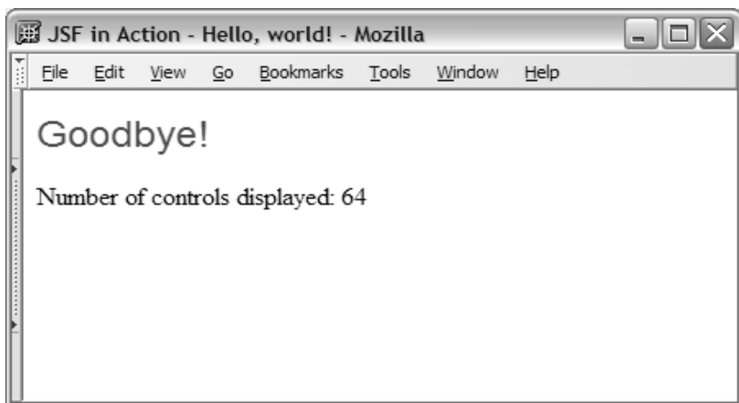
Figure 1.11 The Hello, world! application after you click the Goodbye button. Note that the JavaBean property, which was synchronized with the text box of the first page, is displayed on this page.
