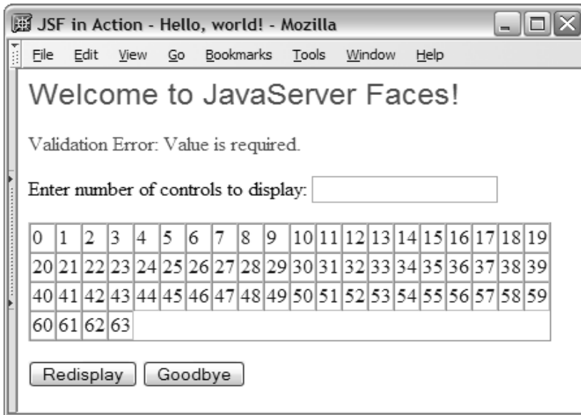
Figure 1.9 The Hello, world! application after you submit a blank value for the required text box field and click the Redisplay button. Because a validation error occurred, the value of the associated JavaBean property didn't change.
