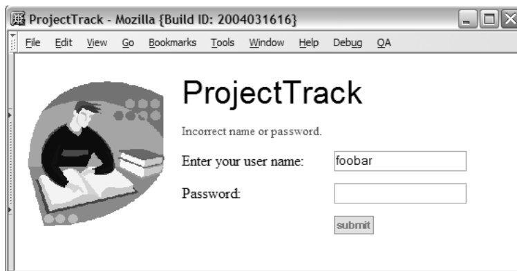
Figure 13.1 The AuthenticationBean.login method returns an error message to the user if no User object can be found.
