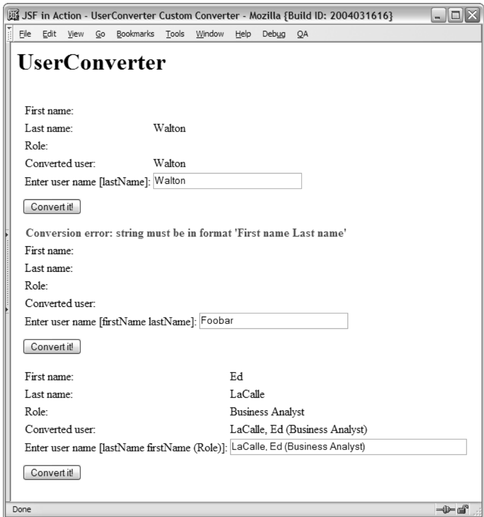
Figure 20.4 The UserConverter converts between a User and a String . This screenshot shows three different styles: last name only (“Walton”), first name and last name (“John Mann”), and last name and first name with the role displayed (“LaCalle, Ed (Business Analyst)”). The second example shows a conversion error because the user entered a value in the wrong format. Note that the value of the user object hasn’t changed, though, because JSF will not update an object with an incorrect value.
