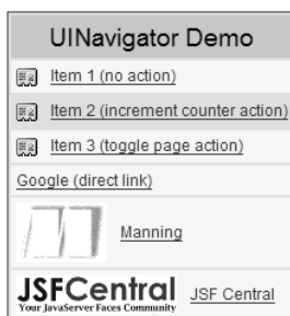
Figure 19.5 UINavigationController with vertical layout, CSS styles, and a combination of items that reference direct links and action methods (the second item is selected).
