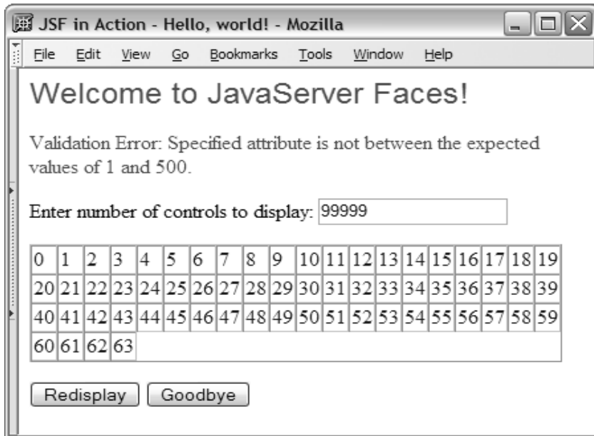
Figure 1.10 The Hello, world! application after you enter in the value "99999" into the text box and click the Redisplay button. The field only accepts numbers between 1 and 500, so a validation error is shown. Because a validation error occurred, the value of the associated JavaBean property didn't change.
