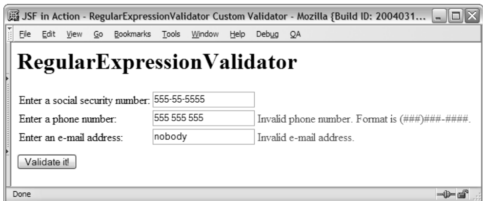
Figure 20.2 The RegularExpressionValidator in action for validating a U.S. social security number, a U.S.-style phone number (with optional area code), and an email address. Error messages can be customized, and displayed via an HtmlMessage or HtmlMessages component.
