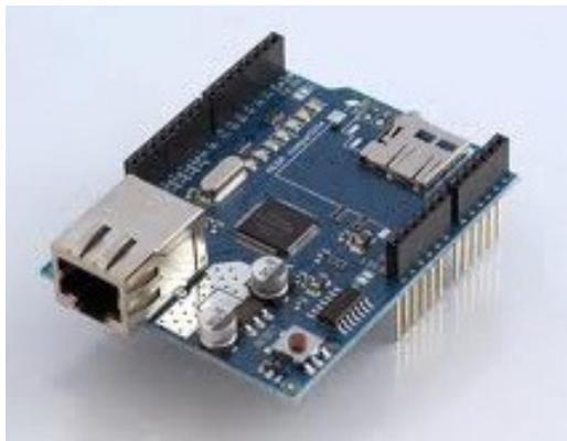
Figura 4: Ethernet Shield.
