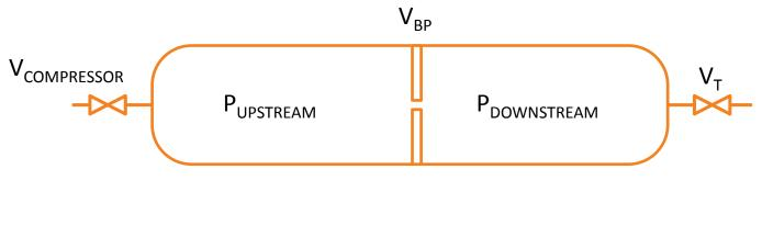
$P_{UPSTREAM} = 50 \text{ PSI}$  $V_T$  opens at time = 15 s  $\Delta P_{REF} = 10 \text{ PSI}$
