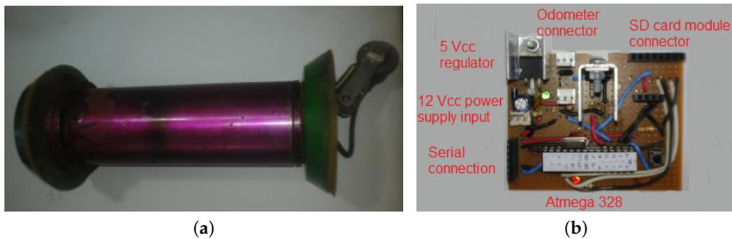
**Figure 5.** Devices used in this work: (a) Prototype PIG; (b) Electronic board. Source: By Authors.
