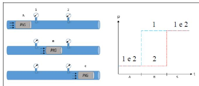
Figure 12. Effect of PIG on the readings of two consecutive pressure sensors. Source: From Freitas [15].
