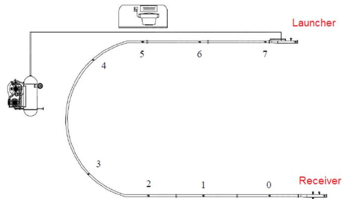
**Figure 7.** Positions of the pressure sensors along the pipeline. Source: By authors.
