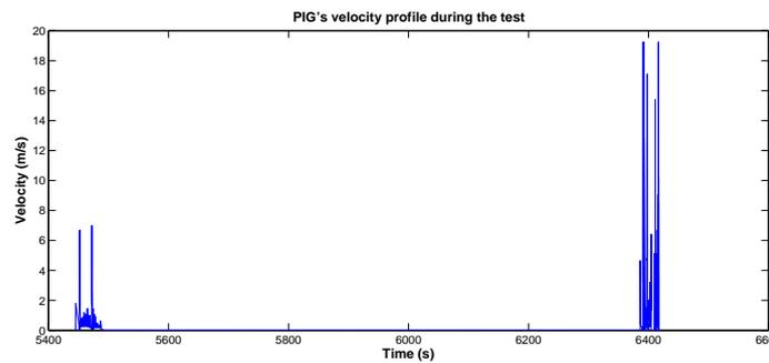
Figure 14. PIG’s velocity profile during the test. Source: By Authors.
