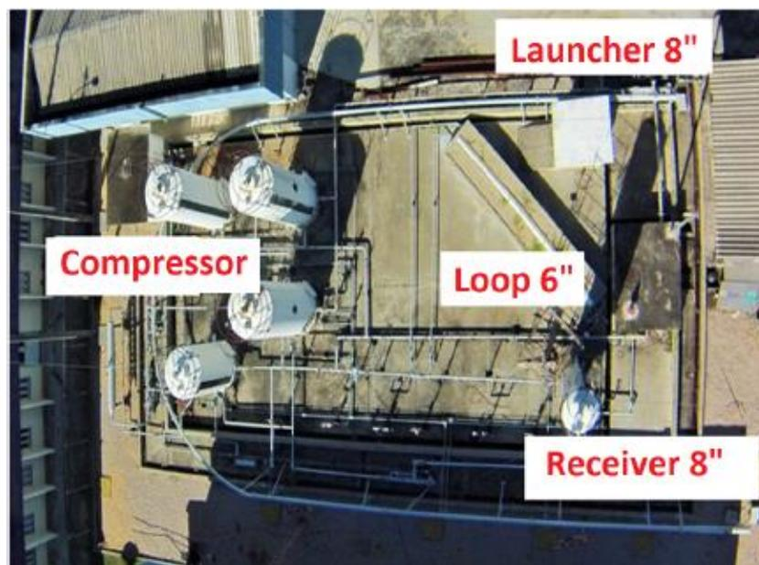
**Figure 6.** Testing Pipeline of 6'' in Upper View. Source: Adapted from Lima et al. [16].
