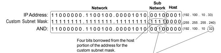
The ANDING process of the four borrowed bits shows which range of IP addresses this particular address will fall into.
