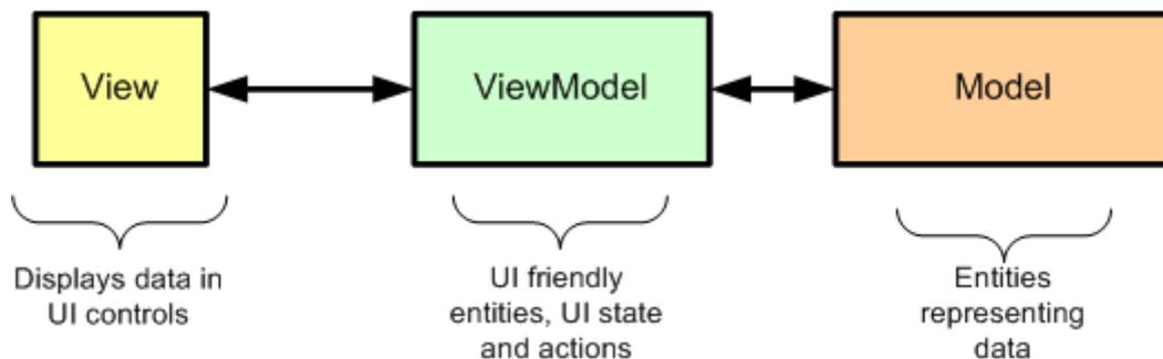
**Figura 4: Model-View-ViewModel Pattern**
