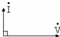
figura 1.6 – Diagrama fasorial circuito C.
